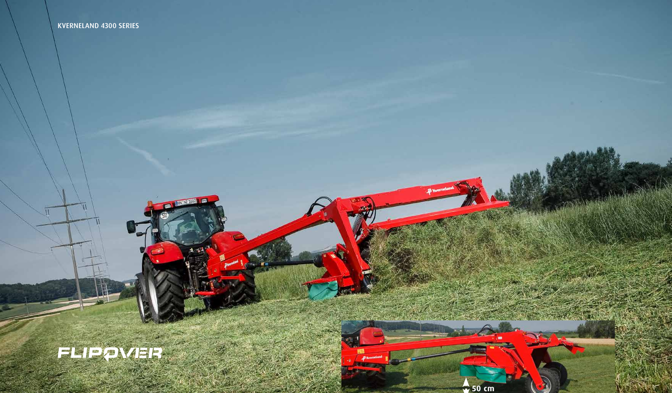
Clearance of 50 cm due to the design of the trolley.
