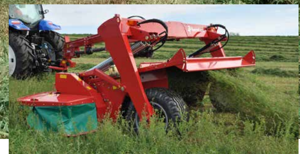
Operation on either left or right side - set from the tractor cab.
