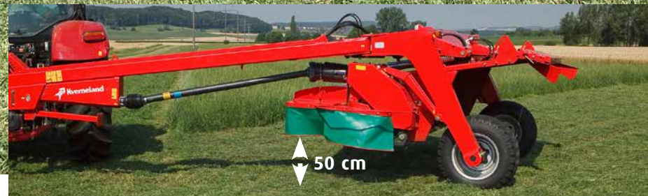
Clearance of 50 cm due to the design of the trolley.
