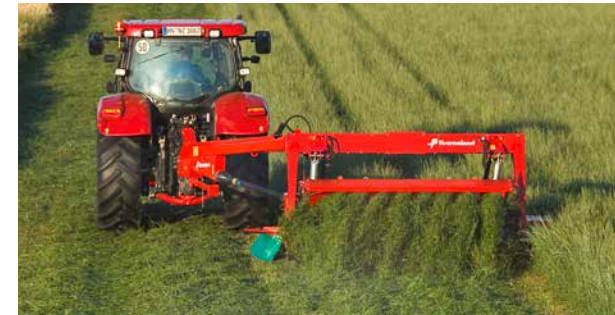
The crop is directed inwards, away from the unmown crop.
