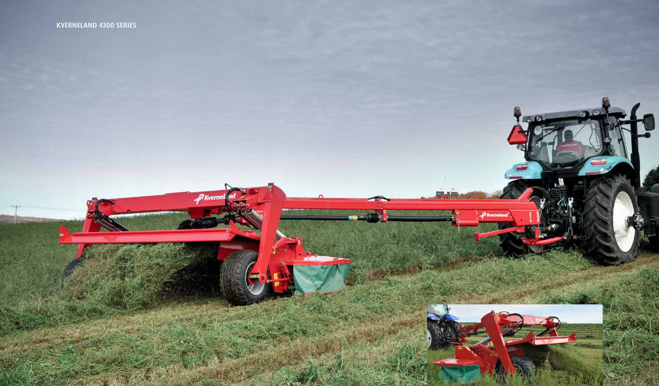
Operation on either left or right side - set from the tractor cab.
